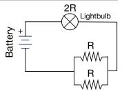
(b) Develop an expression for the voltage drop across the light bulb as a fraction of the battery voltage, V. Give detailed support.
